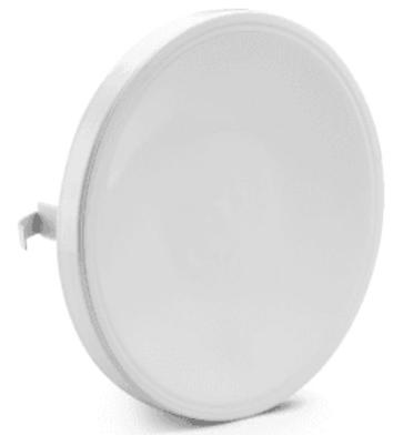
OPT Metal is a round valve with aerodynamically design with good characteristics in terms of noise level, air flow capacity and pressure drop. The valve is mounted in a ceiling or a wall and is intended for ventilation systems with a relatively high pressure drop. The design of the valve and a gasket of moltoprene prevents soiling.
